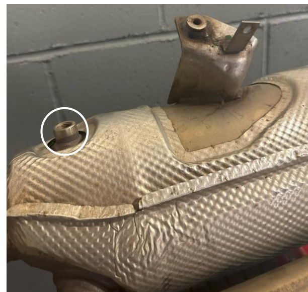
Figure 11v: x1 port at rear of section
