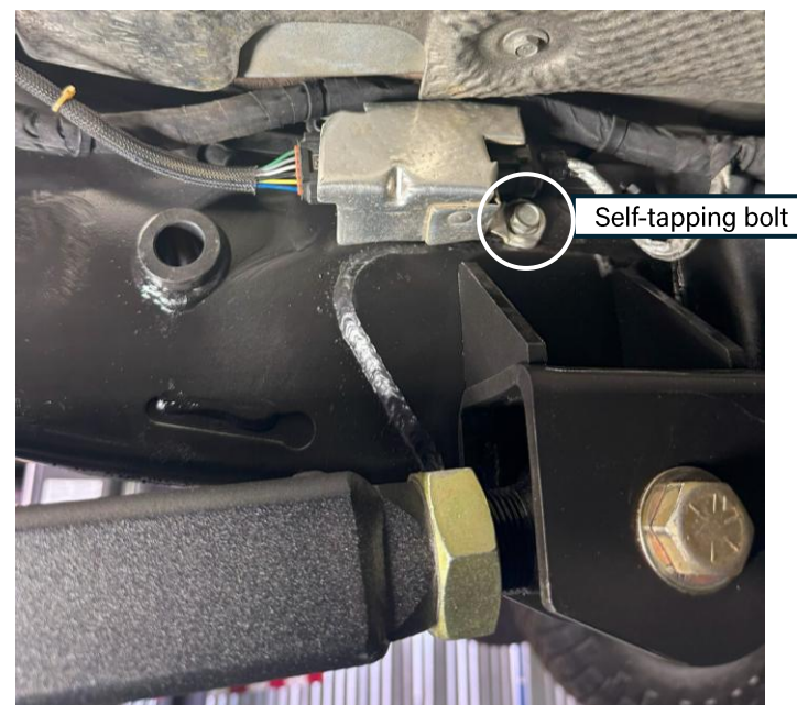
Figure 12c: Sensor relocated with modified heat shield
