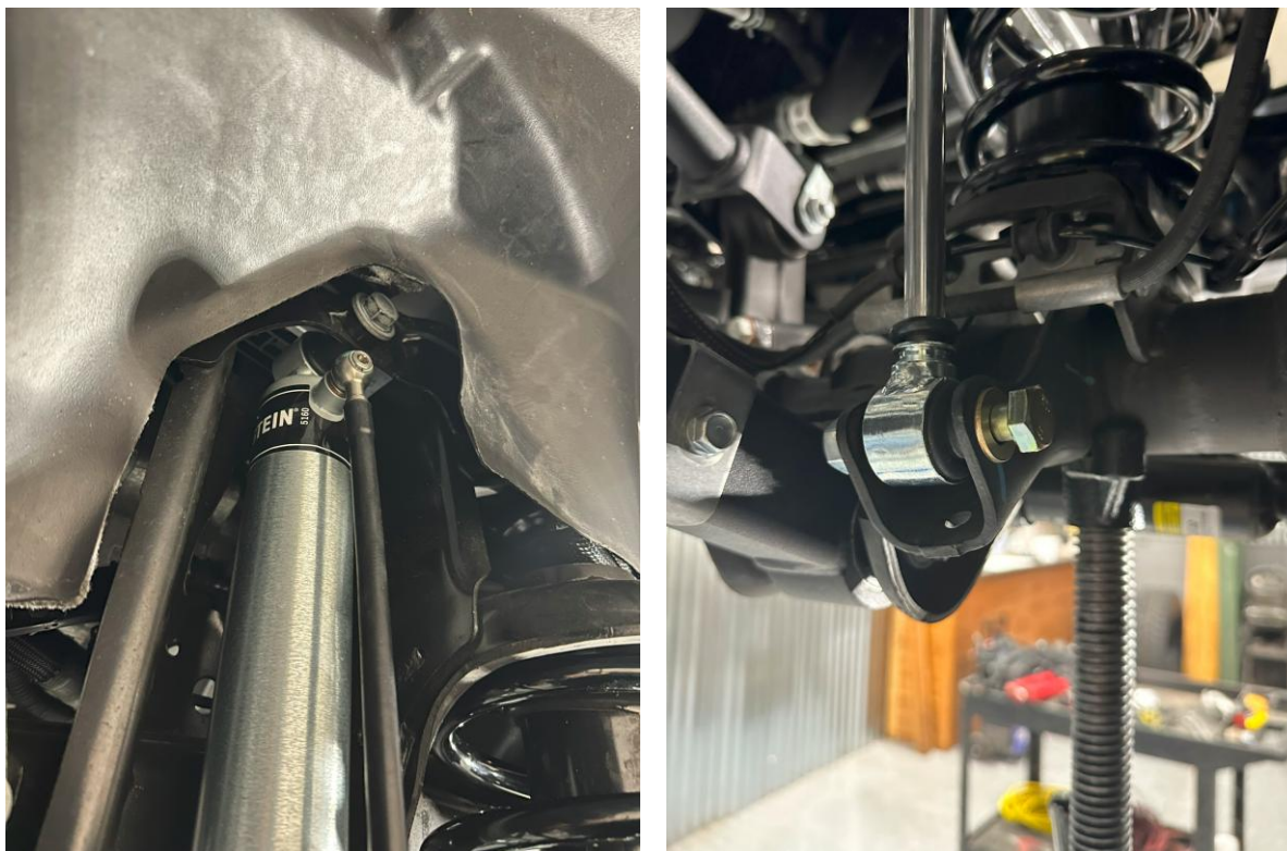
Figure 16: Front shock top and bottom bolt installed loosely
