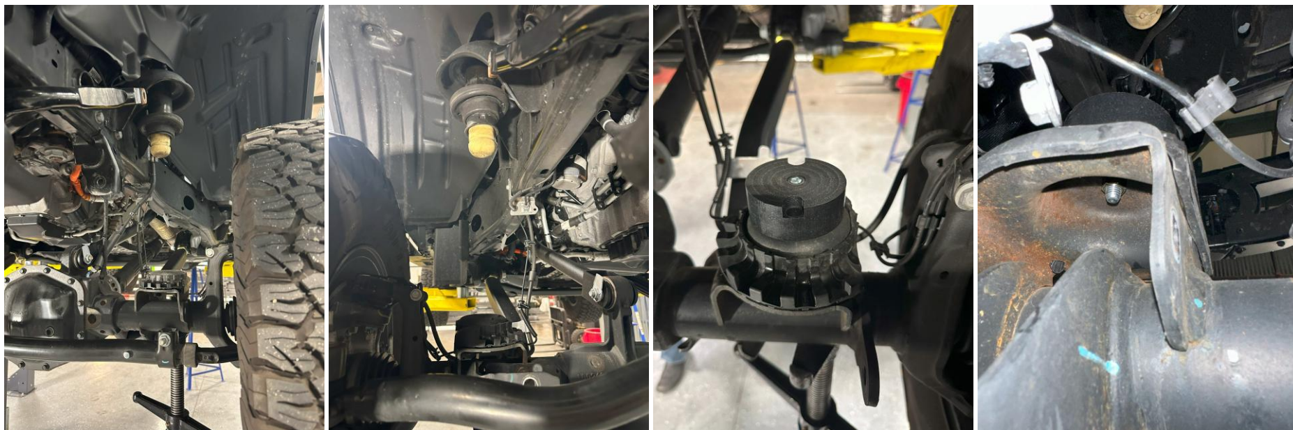
Figure 13: Axle drooped with old springs removed, and bump stops installed
