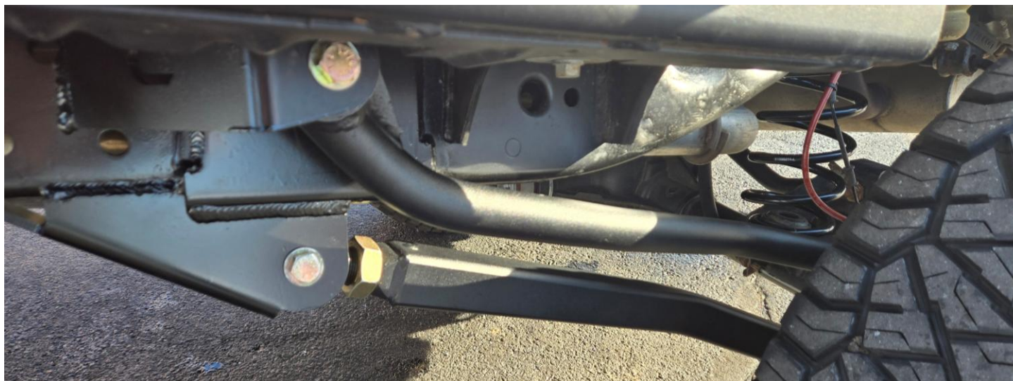
Figure 28: Rear frame brackets and long arms installed
