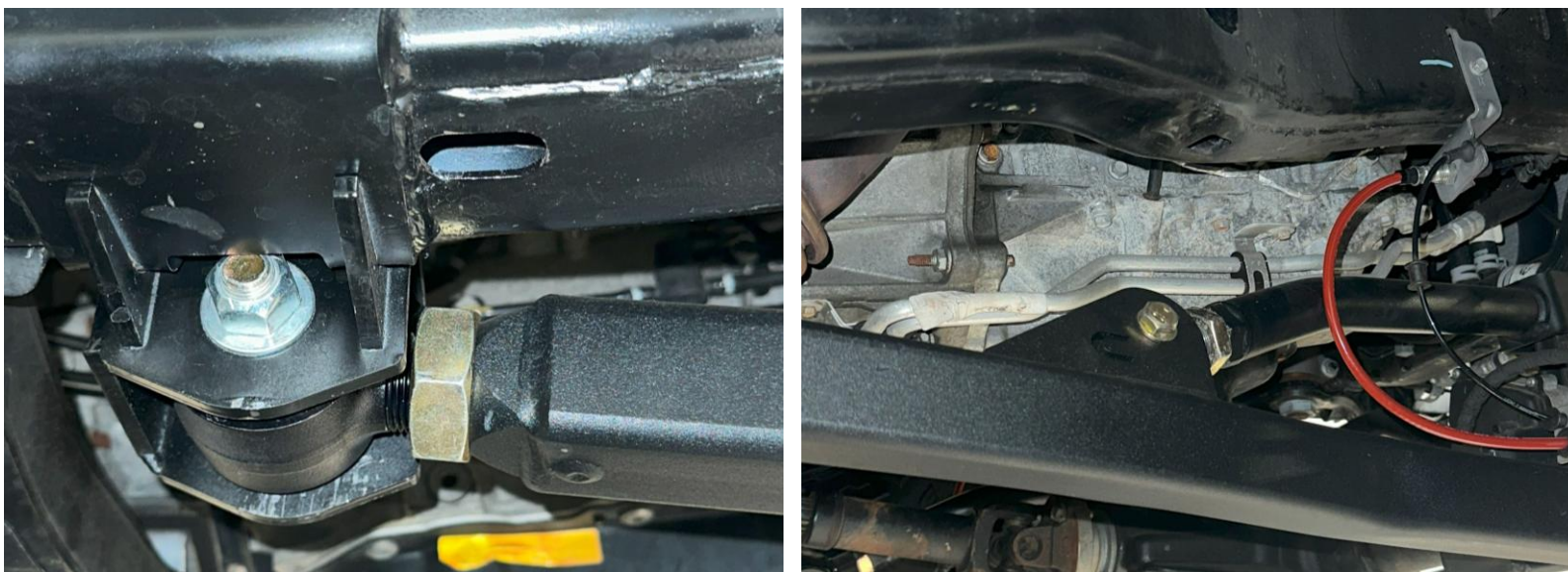
Figure 12: Front frame brackets and long arms installed
