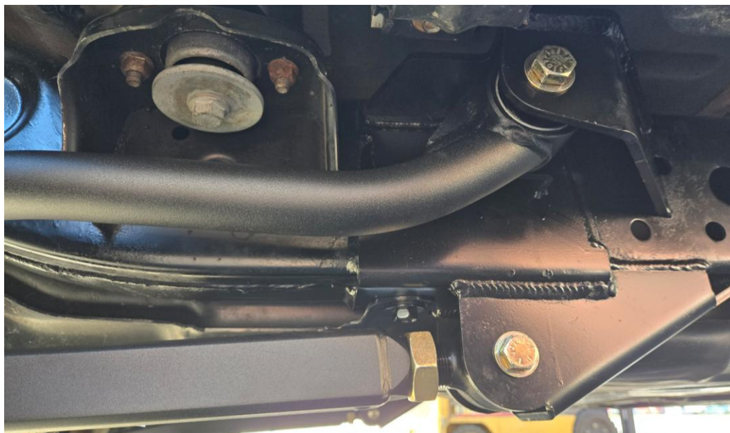
Figure 34: Long arm kit installed
