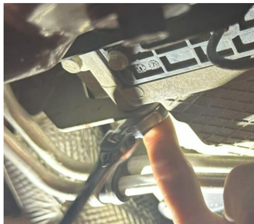
Figure 12s: Front hanger removal
