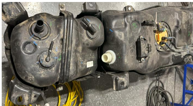
Figure 27b: Diesel gas tank ready to be reinstalled (follow instructions from COR-4810200/5010200)
