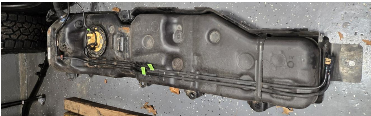
Figure 27: Regular gas tank dropped (follow instructions from COR-5009200/4809200/5009300/4809300)
