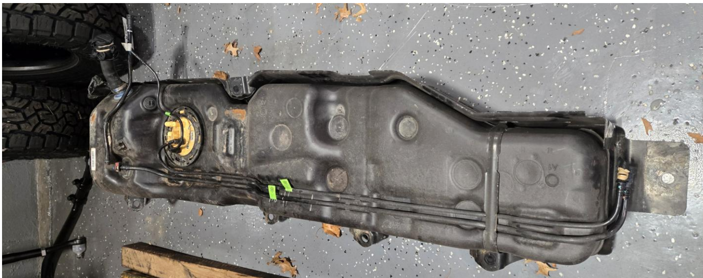
Figure 32: Gas tank ready to be installed back into mounting position
