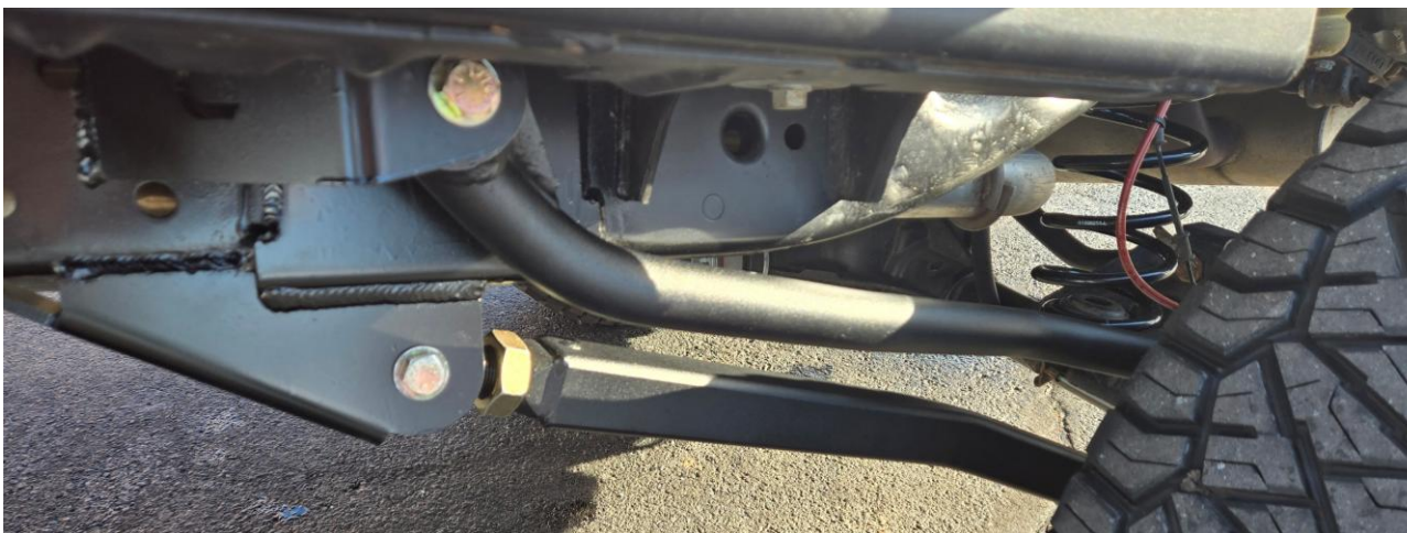
Figure 30: Driver side lower and upper control arms installed
