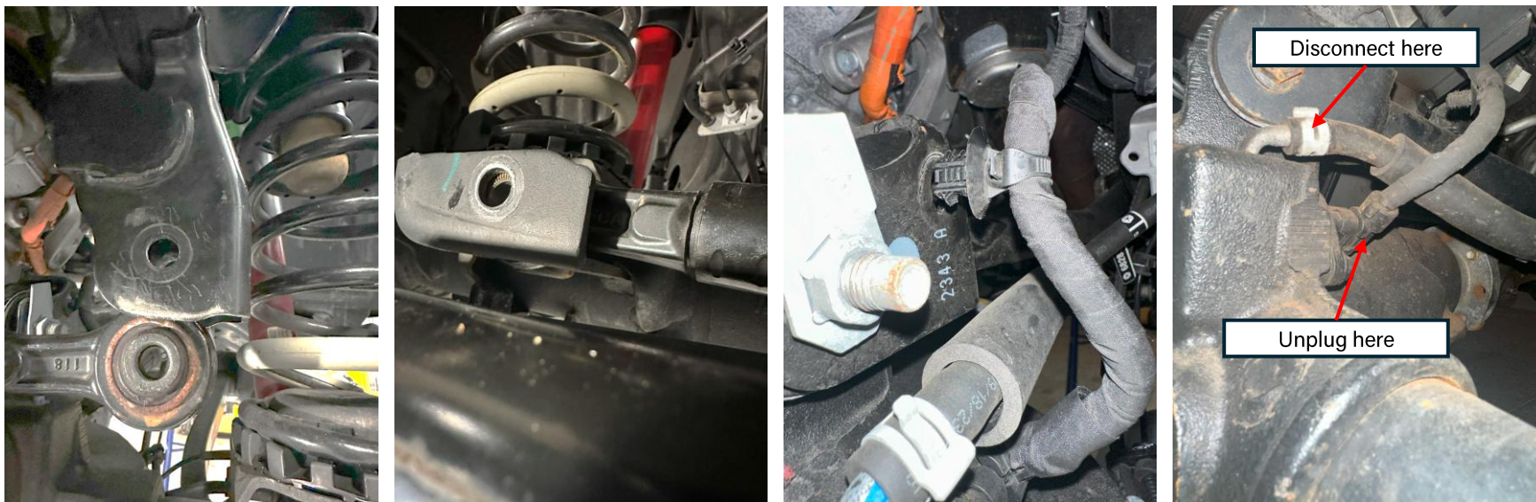
Figure 7: Front factory track bar bolts locations (left) and wiring harness/breather hose and plastic clips (right)
