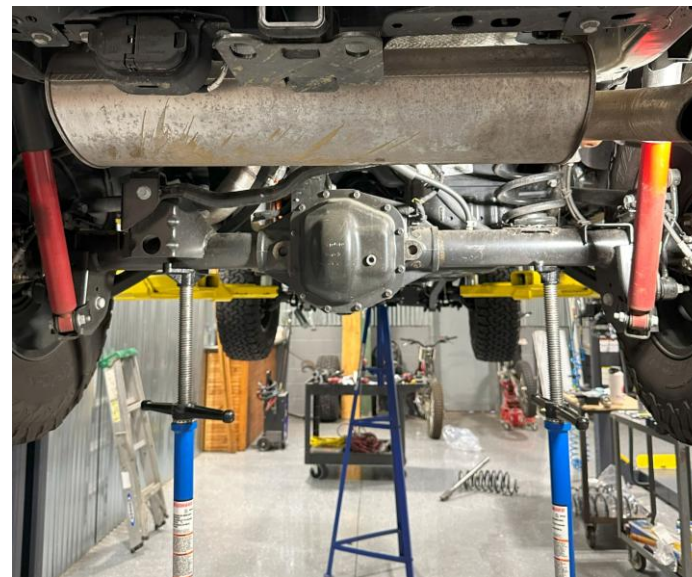
Figure 18: Vehicle rear axle supported by lift and jack stands
