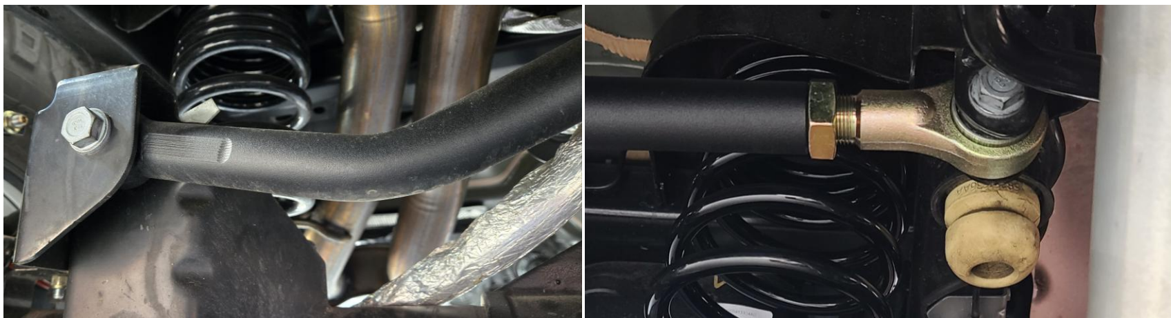
Figure 31: New rear track bar installed
