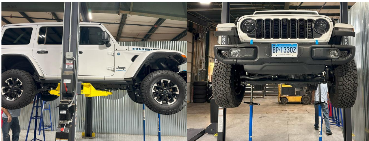
Figure 1: Vehicle supported by lift and jack stands
