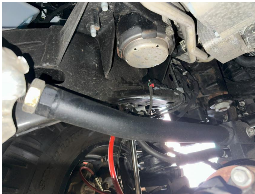
Figure 12: New driver-side upper control arm installed with original hardware
