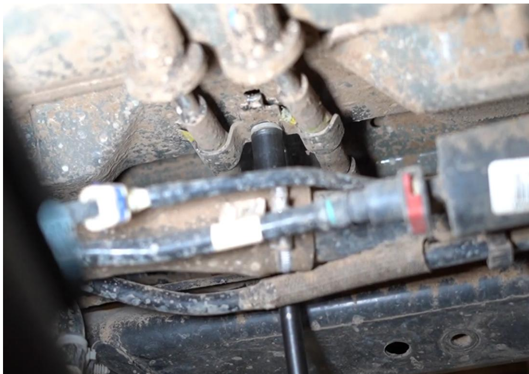
Figure 29: Emergency cable bracket tightened
