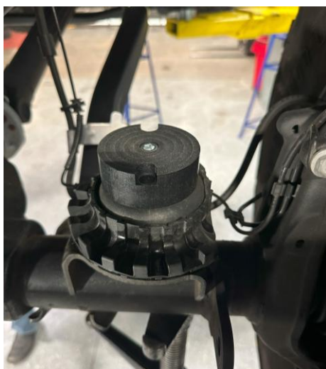
Figure 2: Bump stop installed on front 2018+ JL axle
